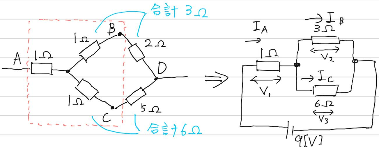
$$I_A = I_B + I_C \quad \dots \textcircled{1}$$
