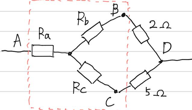
$$\begin{aligned} \text{---} \\ R_a &= \frac{R_2 R_3}{R_1 + R_2 + R_3} = \frac{3 \cdot 3}{3 + 3 + 3} \\ &= 1 [\Omega] \end{aligned}$$
